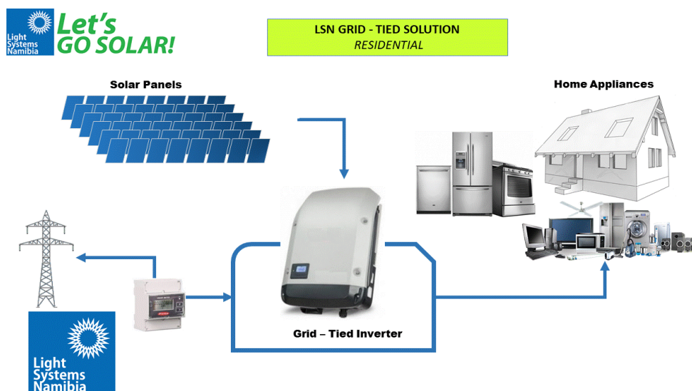
Fig.2 A typical Solar Grid Tied Installation.
